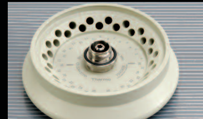
▶ 36 x 0.5 mL rotor with screw-on lid
